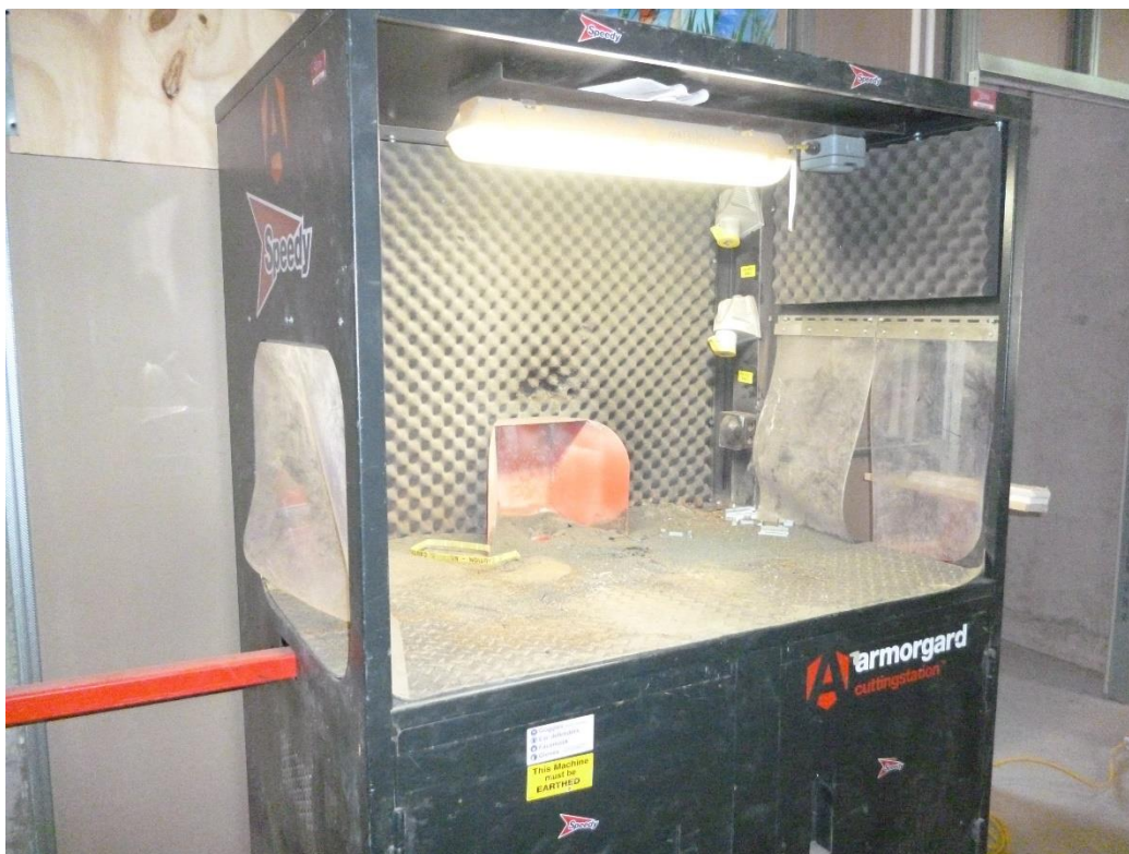
Cutting stations can prevent noise and dust exposures to colleagues working nearby: reducing risk closer to the source and reducing the need for PPE
